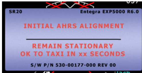
Figure 7. Entegra EXP5000 AHRS Alignment Message
